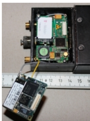
GPS tracker open with SIM card
