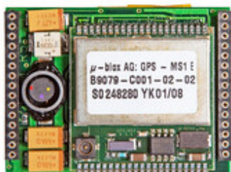
Module providing the GPS signal
