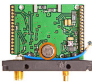
Module providing RF transmission capabilities (other side)
