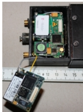
GPS tracker open with SIM card
