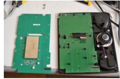
On the left: modified version of the phone largest circuit board (with surveillance device) without the battery pack. On the right: unmodified version.
