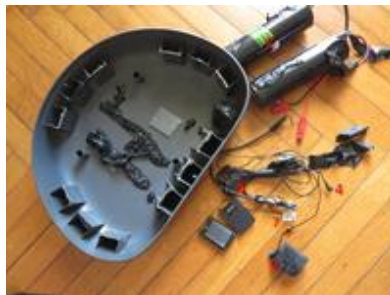
2: two batteries of the listening device ; 4: microphones connected to the listening device ; 6: dismantled listening device ; 7: SD card
