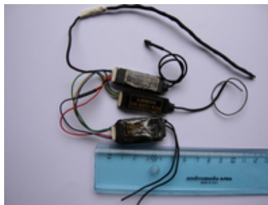
Microphone inside the cooker hood
