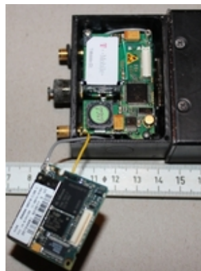
GPS tracker open with SIM card
