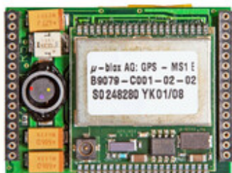
Module providing the GPS signal
