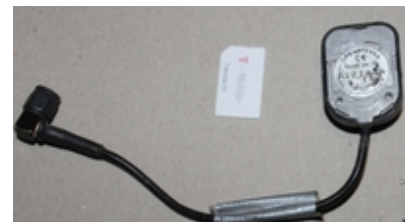
GPS antenna and SIM card
