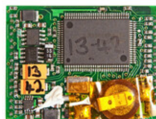
Module providing the GPS signal (other side)
