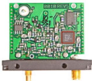
Module providing RF transmission capabilities
