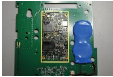
Modified version of the phone largest circuit board, with the cover of the shielded module removed.
