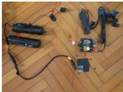
1: control unit ; 2: batteries ; 3: GPS antenna ; 4: microphone ; 5: SIM card
