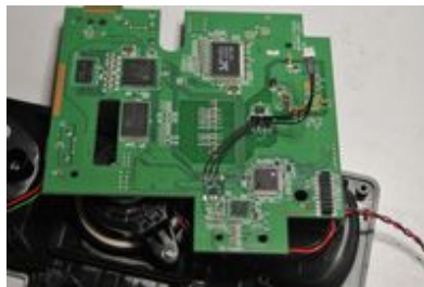
The phone smallest circuit board, with added wiring to allow recording of audio by the surveillance device on the other circuit board.
