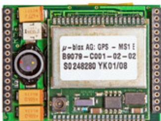
Module providing the GPS signal
