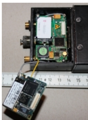
GPS tracker open with SIM card
