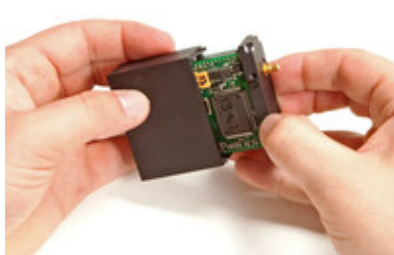
Transmitter-receiver module (open)
