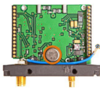
Module providing RF transmission capabilities (other side)
