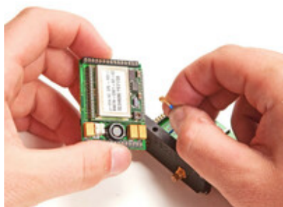
Transmitter-receiver module (open)
