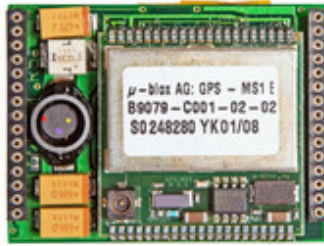
Module providing the GPS signal
