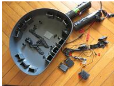
2: two batteries of the listening device ; 4: microphones connected to the listening device ; 6: dismantled listening device ; 7: SD card
