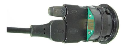
The Dongle 3 cable can be used to download and configure the recorder using Whisper2.
