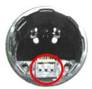
2. Line up the recorder so that the three gold pads will contact the pins
