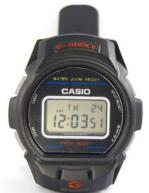
The Geonautics A3w concealment contains an A3 audio recorder in a watch, for the purpose of recording conversations during meetings etc. with its internal microphone.
