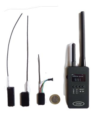
Such technology is detached in a totally different way from the transmission systems employing similar modulations in FSK or GMSK for which, at the same rf power, consumption are around 10-15 times higher, thereby limiting the duration of a monitoring system powered by battery.
