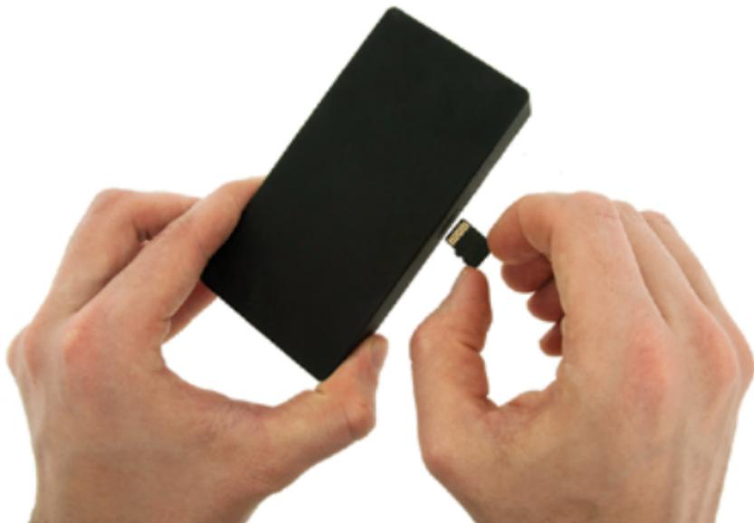
To install the micro SD card, place the camera on a flat surface with the BrickHouse Security logo facing upwards. The card should be inserted with the gold contacts facing down, away from the logo.
